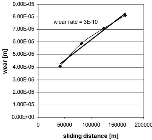
Figure 9 Overall brush wear vs. sliding distance.
