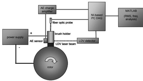
**Figure 4 Schematic of homopolar motor with DAQ system**
