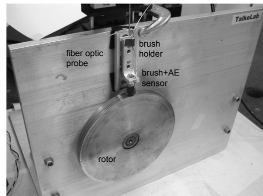
Figure 3 Homopolar Motor Test Rig
