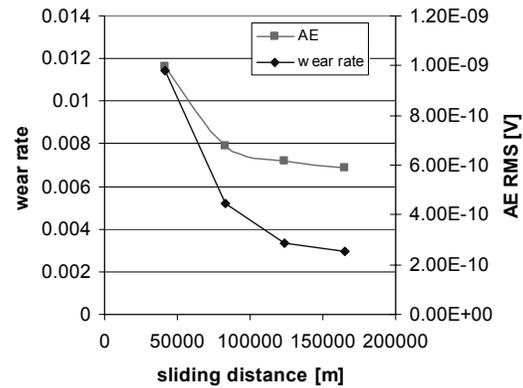
Figure 10 Brush wear-rate monitoring with AE RMS.
