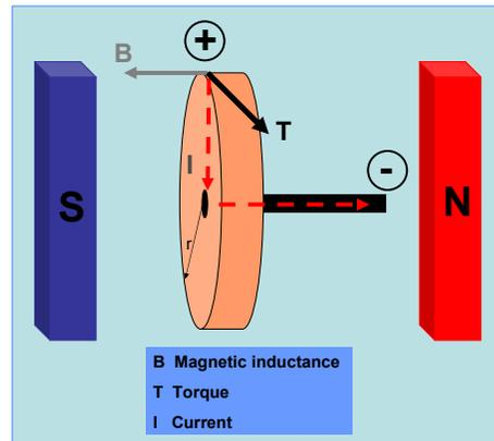
Figure 1 Schematic of homopolar motor
