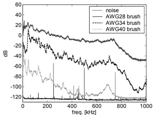
**Figure 6 AE Spectral density variation with brush type**
