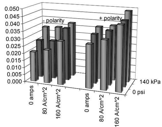
**Figure 8** AE RMS values for full-factorial parameter testing on full-scale test rig.
