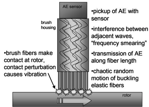
Figure 2 AE Sources at the Brush/Rotor Interface
