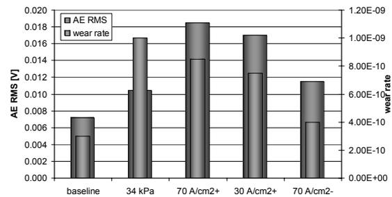
Figure 11 AE RMS and wear rates under different operating conditions.
