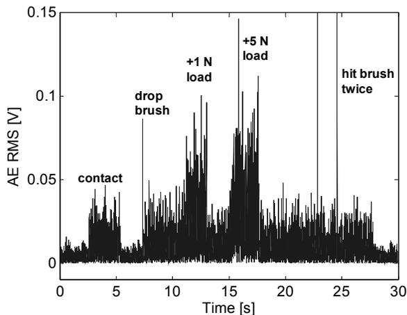
**Figure 7** Brush contact monitoring with AE RMS signal.
